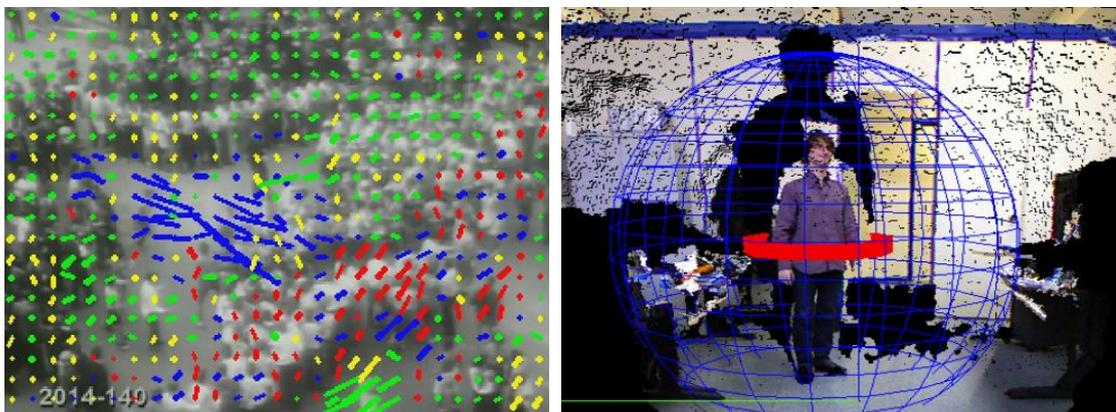
Figure 1: Left image: low-level features extracted from a large group of moving people using optical flow algorithms, Right image: mid-level features: 3D personal spaces around a user acquired using the Kinect 3D camera [10].
